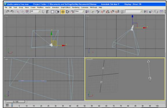
Fig. 5. Generation of synthetic data (images with known calibration parameters and object geometry) with 3D Studio Max.
