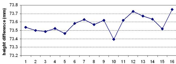
Fig. 6. The same difference in elevation measured by placing the camera at different stations. The standard deviation of the values shows a discrepancy between the measurements of  $\pm 0.1$  mm.
