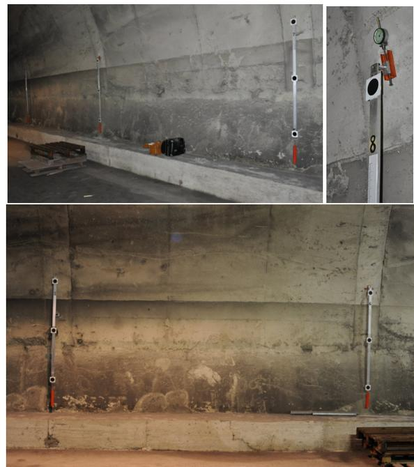
Fig. 8. The experiment in a real tunnel with a sequence of rods on fixed and movable benchmarks.
