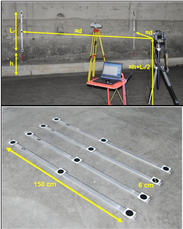
Fig. 2. An example of the basic operational scheme of photogrammetric leveling with two rods placed on benchmarks and a digital camera (top), along with some examples of the special targeted rods (bottom).
