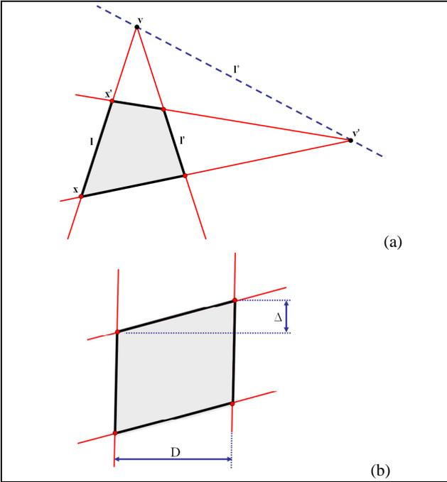
Fig. 3. Geometric quantities used to rectify the original image (a) and the estimated values (b).
