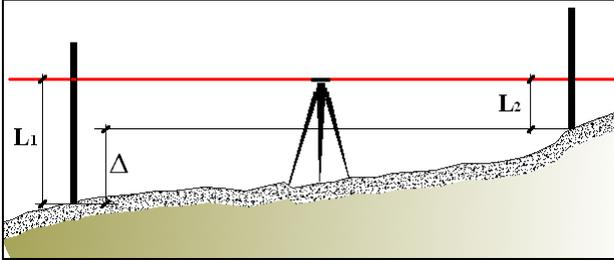
Fig. 1. Basic principle of geometric leveling: the difference in elevation can be estimated with a difference of readings.
