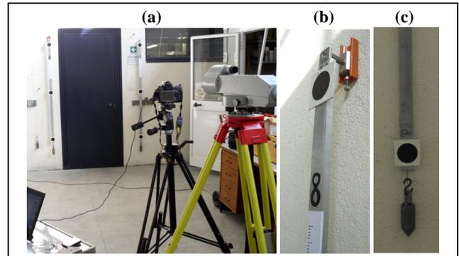
Fig. 7. The test with an optical level: (a) the rod with a graduated card mounted on a movable benchmark (b) and a heavy weight to make each rod more stable (c).
