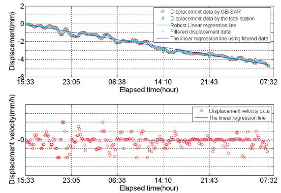
Fig 9. Displacement and velocity time series of point 3
