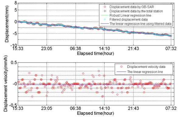
Fig 8. Displacement and velocity time series of point 2
