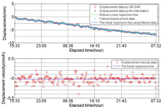
Fig 7. Displacement and velocity time series of point 1
