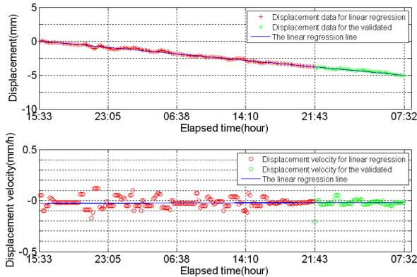
Fig 6. Displacement and velocity time series of the main slip
