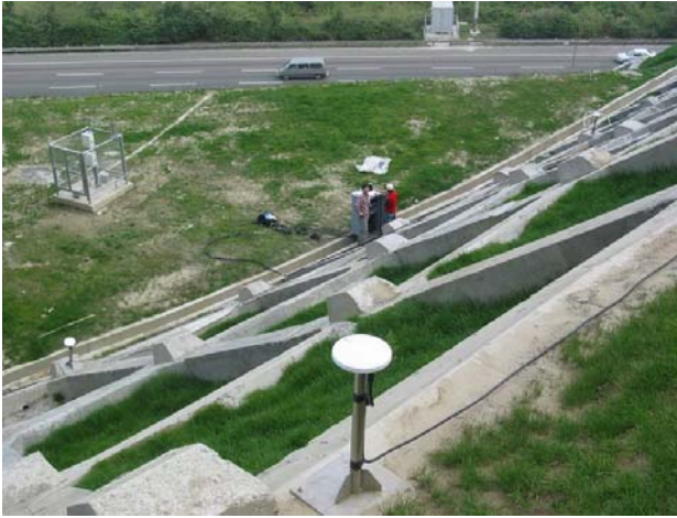
Figure 3. Experimental area and multi-antenna GPS system
