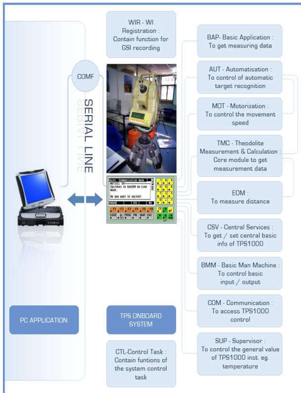
Figure 1: Client/Server Applications and GeoCOM Function
