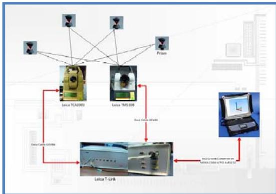
Figure 2: Communication between computer unit and sensors
